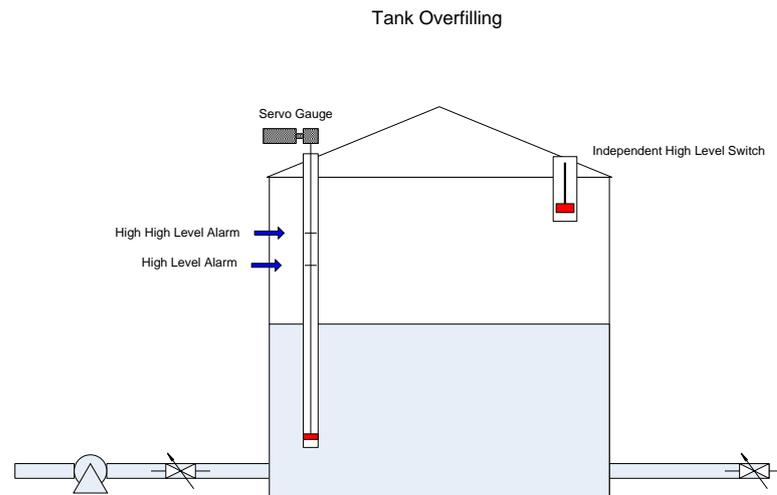
The risk to a loss of containment is – failure to correctly manage the liquid level in the tank.
